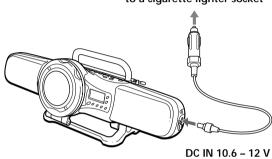
To replace the fuse of the car battery cord Be sure to use the fuse with the correct amperage. (4 A, 125 V, length 31.75 mm)
